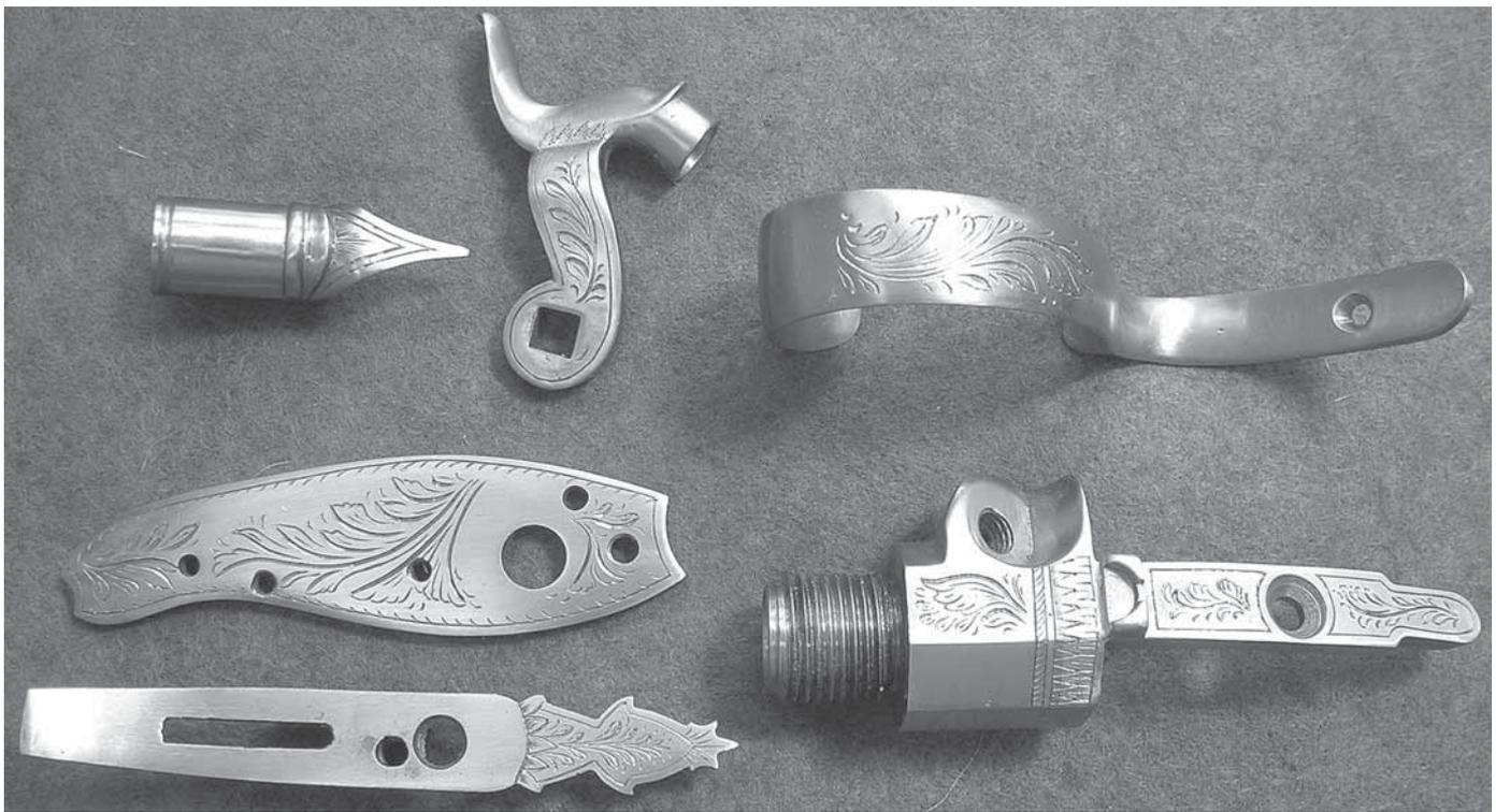
Figure 8 – Engraved parts with rough engraving done on imported belt pistols of 1800's.
